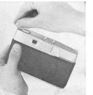
direction of the arrow mark. This action will wind film back into its safety cartridge.
